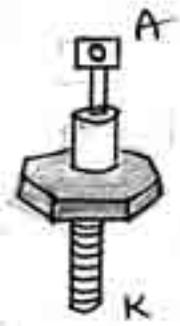
Fig ③: High current diode
